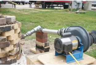
Figure 3- Furnace air supply equipment
